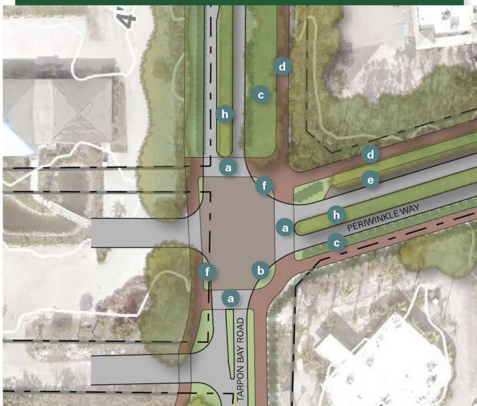
Figure 51: Option 2, protected intersection alternative with turn lanes replaced by medians, reducing unnecessary pavement and providing a refuge space for pedestrians.
