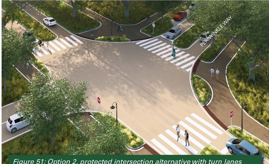
Figure 51: Option 2, protected intersection alternative with turn lanes replaced by medians, reducing unnecessary pavement and providing a refuge space for pedestrians.
